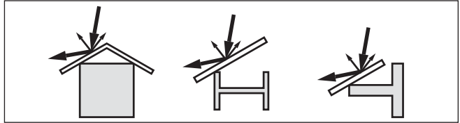
Fig. 29: Cover flat, large-area profiles with deflectors
